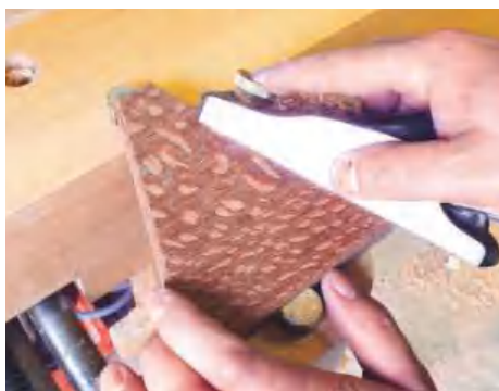
A decent chamfer on the edge prevents the lacewood from chipping
